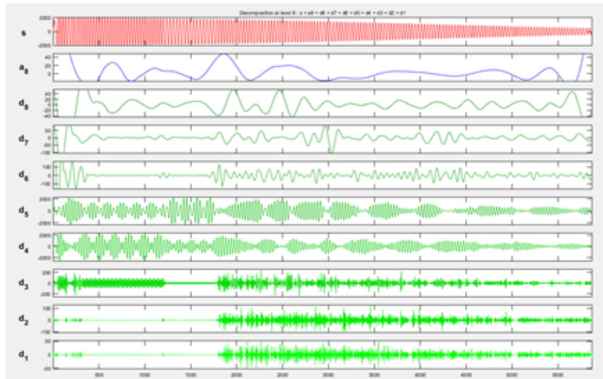
Fig. 7. Wavelet Daubechies Level 8 Medium Voltage Motor 13800 V, 3 MVA; shows the spectrum of the motor with insulation failure for 200kΩ.
