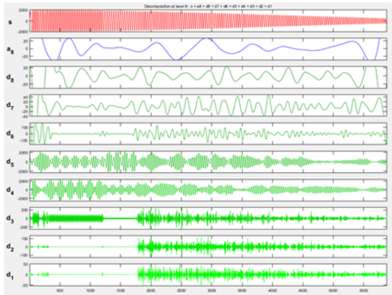
Fig. 6. Wavelet Daubechies Level 8 Medium Voltage Motor 13800 V, 3 MVA; shows the spectrum of the engine in healthy state.
