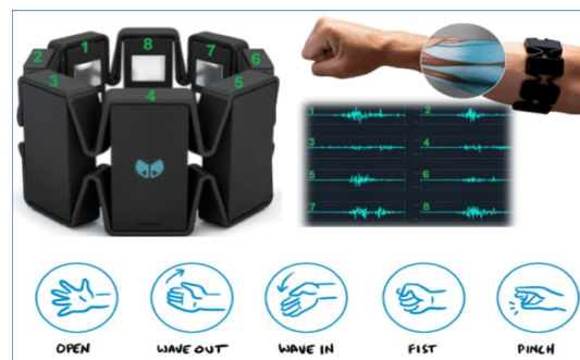
Fig. 6. Myo bracelet with the movements it recognizes in the user.
