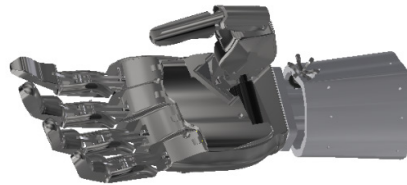
Fig.1. 7DOF hand prosthesis prototype
