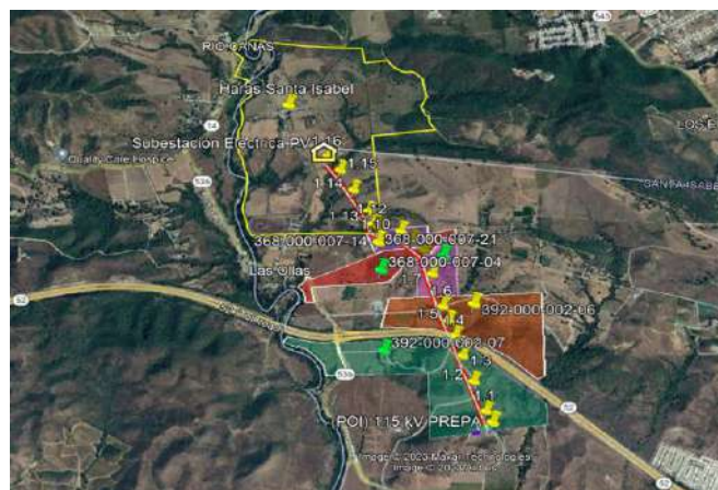
Fig. 15. Route of the 115 kV transmission line from the Juana Díaz land to the point of interconnection. Source: own.
